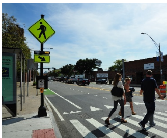
Rectangular Rapid Flashing Beacon (RRFB)
